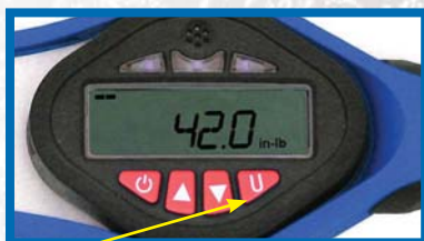
The "U" button changes the units from ft.lb. to in.lb. to Nm to Kgcm.
