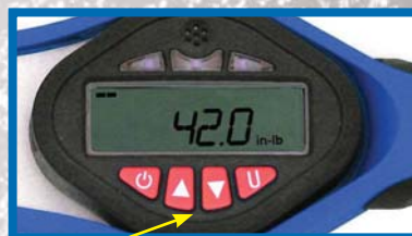
The up and down arrow buttons change the torque value up or down.
